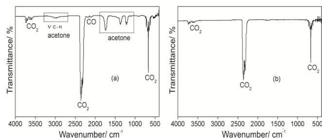
**Figure 4.** FT-IR spectra of gaseous products evolved during the thermal decomposition of lanthanum malonate, as representative of the all compounds, between (a) 573 – 673 K and (b) 673-1000.
