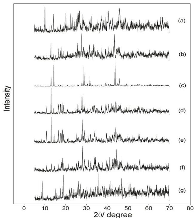
**Figure 1.** X-ray powder diffraction patterns of the compounds: (a)  $\text{La}_2(\text{L})_3 \cdot 4.5\text{H}_2\text{O}$ , (b)  $\text{Ce}_2(\text{L})_3 \cdot 4.5\text{H}_2\text{O}$ , (c)  $\text{Pr}_2(\text{L})_3 \cdot 6\text{H}_2\text{O}$ , (d)  $\text{Nd}_2(\text{L})_3 \cdot 6\text{H}_2\text{O}$ , (e)  $\text{Sm}_2(\text{L})_3 \cdot 6\text{H}_2\text{O}$ , (f)  $\text{Eu}_2(\text{L})_3 \cdot 6\text{H}_2\text{O}$  and (g)  $\text{Gd}_2(\text{L})_3 \cdot 7\text{H}_2\text{O}$ . (L= malonate).
