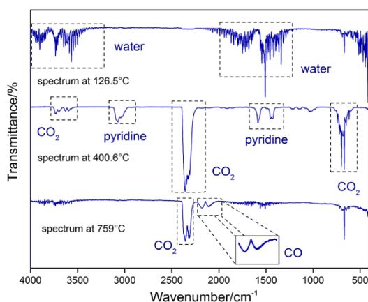
**Figure 4.** IR spectra of the gaseous products evolved during the thermal decomposition of cobalt compound:  $Co(L)_2 \cdot 4H_2O$ , as representative all the nicotinate compounds studied in this work.
