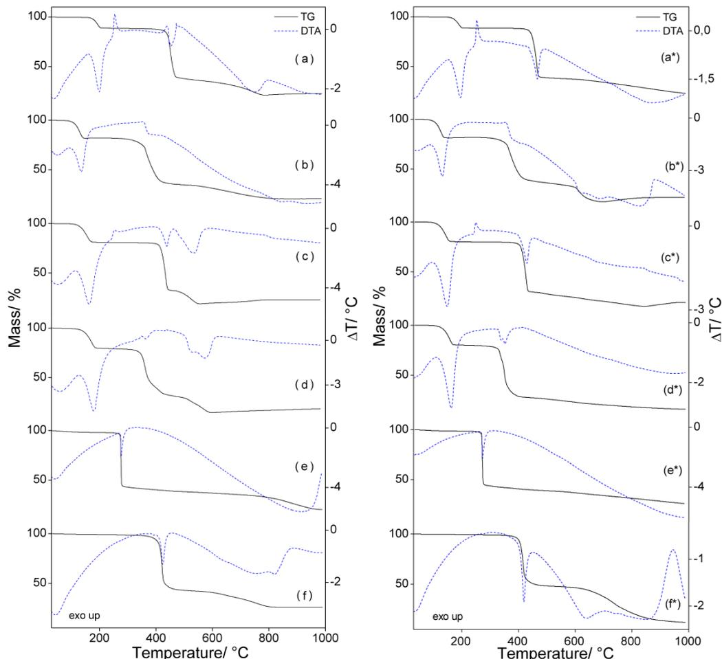
**Figure 3.** Simultaneous TG-DTA curves of the synthesized compounds in (a-f)  $CO_2$  (sample masses: Mn = 7.0602 mg, Fe = 7.0283 mg, Co = 7.0929 mg, Ni = 7.0076 mg, Cu = 6.9630 mg and Zn = 7.0297 mg) and (a-f\*)  $N_2$  atmospheres (sample masses: Mn = 7.0044 mg, Fe = 7.0526 mg, Co = 7.0397 mg, Ni = 7.0193 mg, Cu = 7.0792 mg and Zn = 7.0102 mg).
