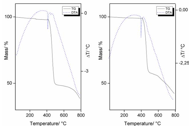
**Figure 2.** Simultaneous TG-DTA curves of sodium nicotinate in (a) CO<sub>2</sub> (m = 3.0527 mg) and (a\*) N<sub>2</sub> atmospheres (m = 3.2556 mg).
